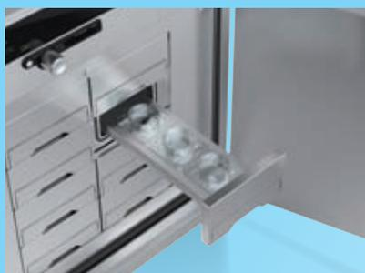
Minimal recovery times achieved by cultivating the Petri dishes in separate slide-in units
