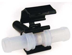
This model is developed to perform a fast exchange of the flow tube (for hygienic reasons e.g. in pharmaceutical industry). The flow meter is suitable for clear and opaque, neutral, corrosive and aggressive liquids, fuel and for periodic monitoring. The flow tube is assembled in the flow system. For measurement and calibration the easy- to- remove housing is placed around the tube and measuring can take place.
