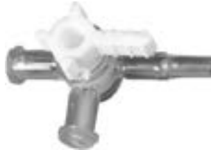
VPB1000062N (Polycarbonate Body with Polyethylene Handle) Three Way Stopcock, (2) Female Luer Thread Style and Male Slip Luer
